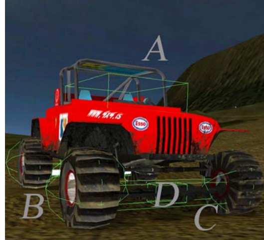
Figure 3: The trained vehicle. Green line surrounding all items representing a primitive building blocks
